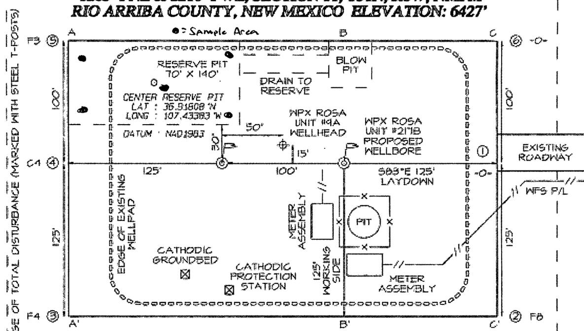
Steel T-Posts have been set to define the Edge of Disturbance limits which are 50' offset from the edge of the staked wellpad.
