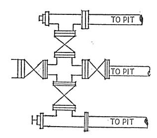
(iii) line will be minimum 2" diameter and have ? valves une of which shall be a minimum 2" check valve
