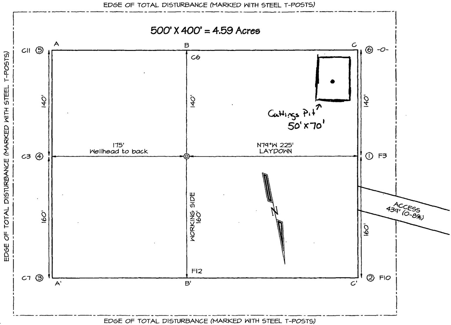
Steel T-Posts have been set to define the Edge of Disturbance limits which are 50' offset from the edge of the staked wellpad.
