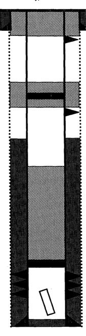
8.625" 24#, J-55 Casing set @ 101' Cement with 80 sxs (Circulated to Surface)
