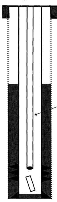
8.625" 24#, J-55 Casing set @ 101' Cement with 80 sxs (Circulated to Surface)
