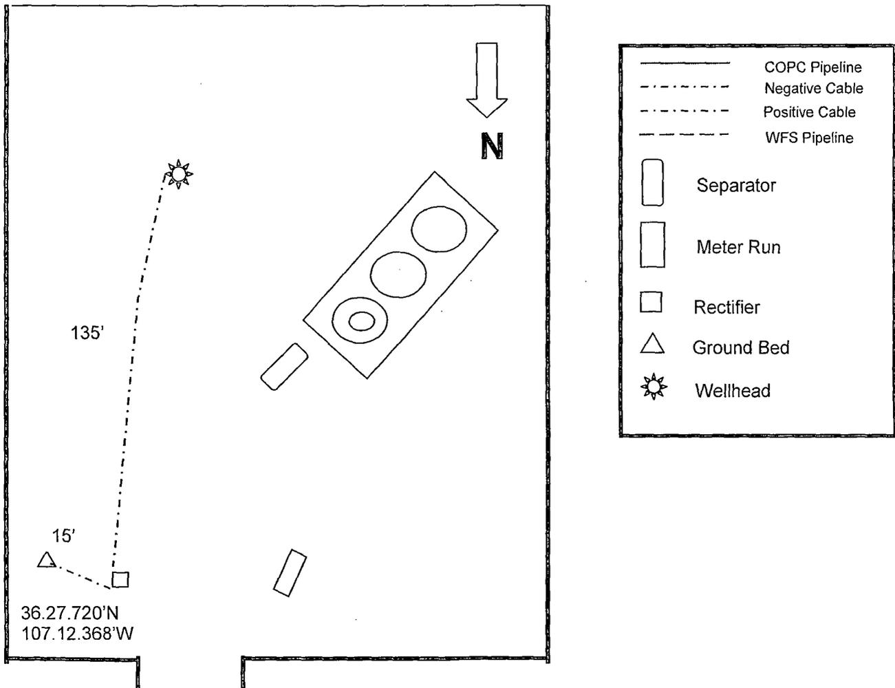
Drill ground bed approximately 135' North East of Jicarilla B #8A wellhead at staked location. Install single well solar at staked location and install cable to new ground bed and to Jicarilla B #8A wellhead at lengths below.
