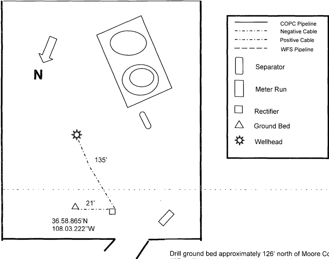
Drill ground bed approximately 126' north of Moore Com LS #3P wellhead at staked location. Install single well solar at staked location. Install cable to new ground bed and to #3P wellhead at lengths below.
