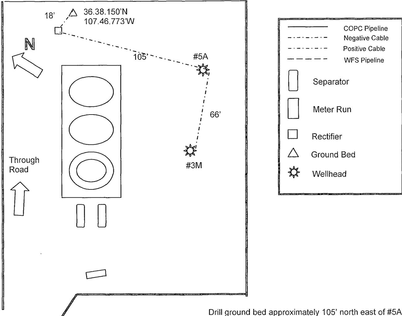
Drill ground bed approximately 105' north east of #5A well head at staked location. Install a dual well solar CP at staked location. Install cable to new ground bed and to #5A and #3M wellheads at lengths below.
