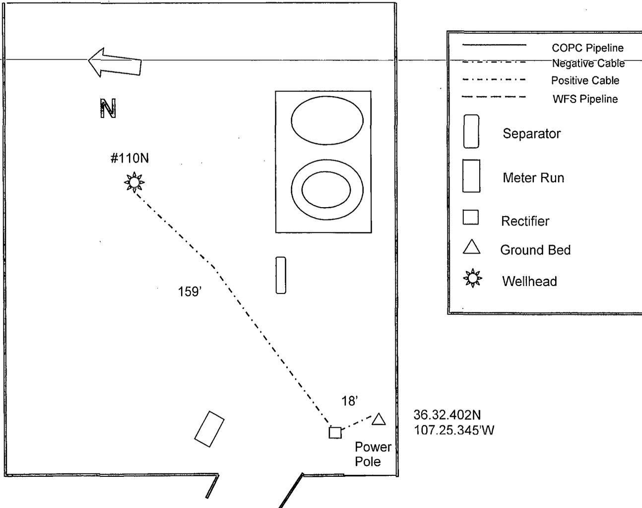
Drill ground bed approximately 162' south west of #110N well head at staked location. Install 40-16 rectifier and meter pole at staked location. We will need a transformer set on Jamez Electric pole #04042 connect to the meter pole and set a meter. Install cable to new ground bed and to the #110N wellhead at lengths below.
