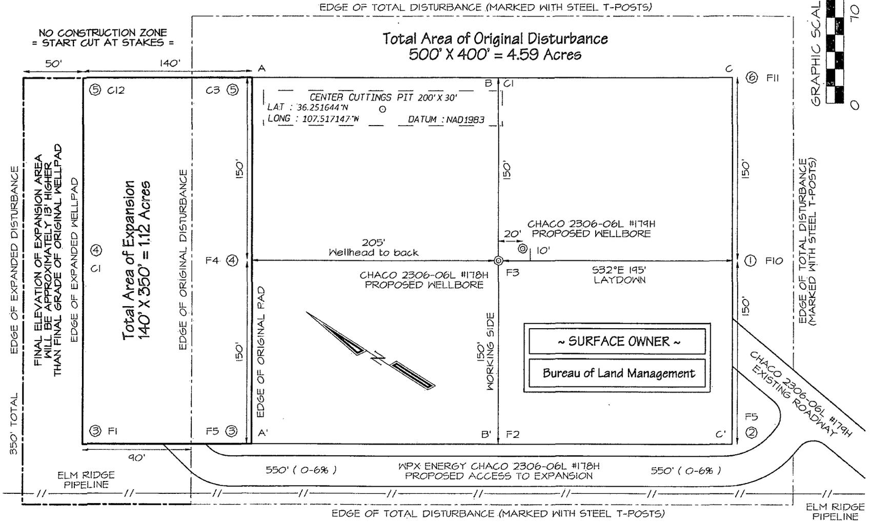
Steel T-Posts have been set to define the Edge of Disturbance limits which are 50' offset from the edge of the staked wellpad.
