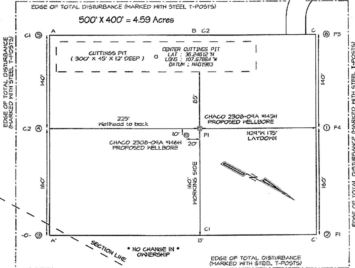
Steel T-Posts have been set to define the Edge of Disturbance limits which are 50' offset from the edge of the stacked wellhead.
