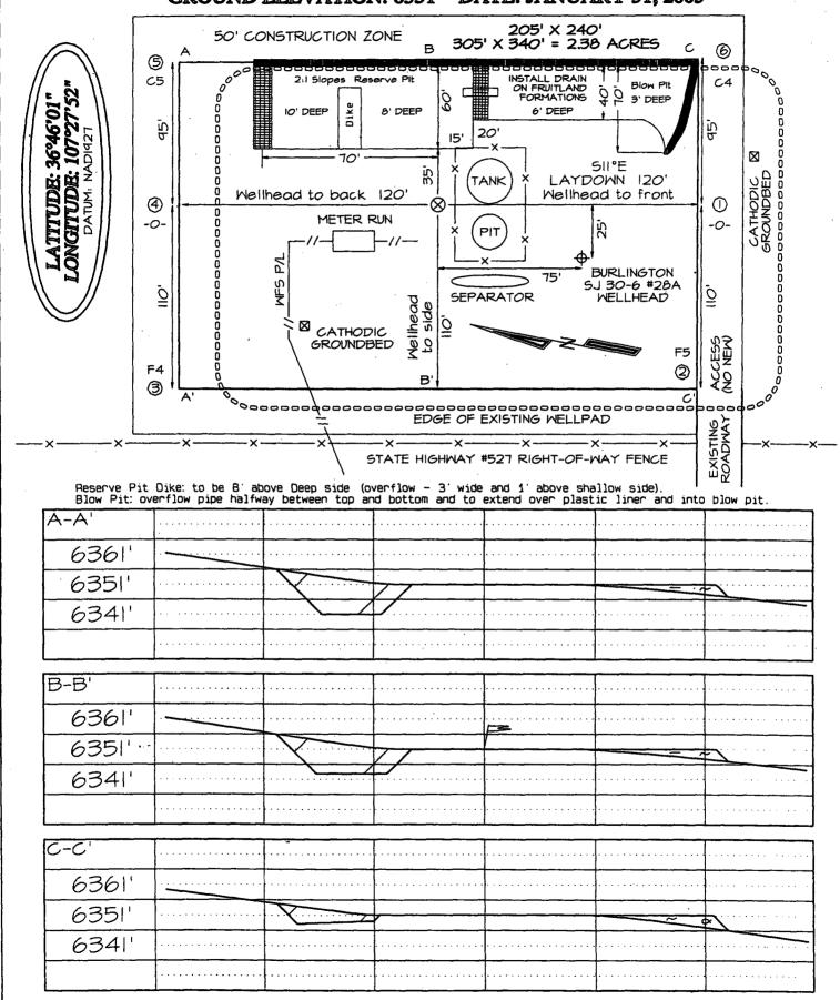
Note: Contractor should call One-Call for location of any marked or unmarked buried pipelines or cables
