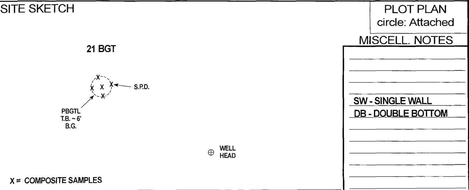
NOTES: BGT = BELOW-GRADE TANK; E.D. = EXCAVATION DEPRESSION; B.G. = BELOW GRADE; B = BELOW; T.H. = TEST HOLE; ~ = APPROX.;
