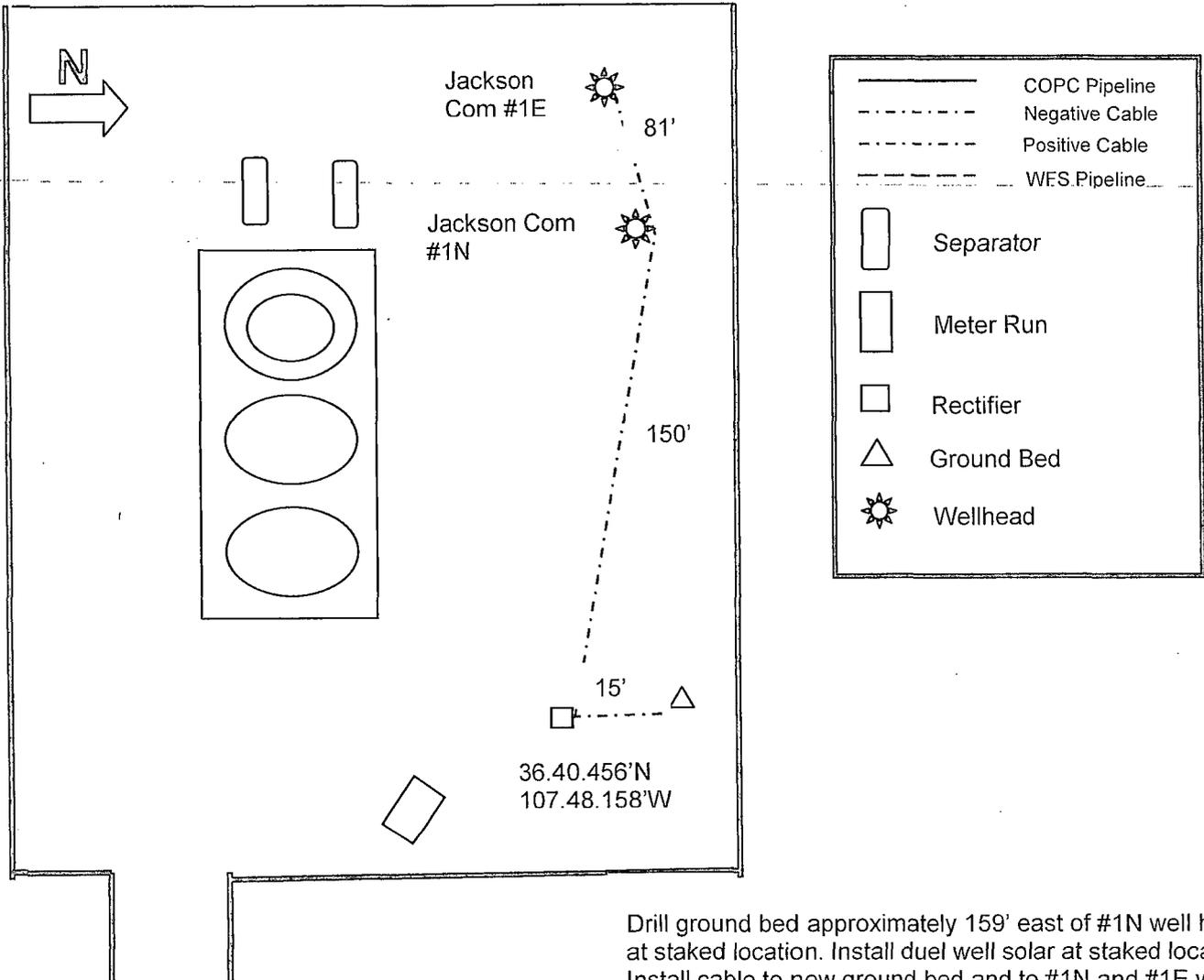
Drill ground bed approximately 159' east of #1N well head at staked location. Install dual well solar at staked location. Install cable to new ground bed and to #1N and #1E well heads at lengths below.
