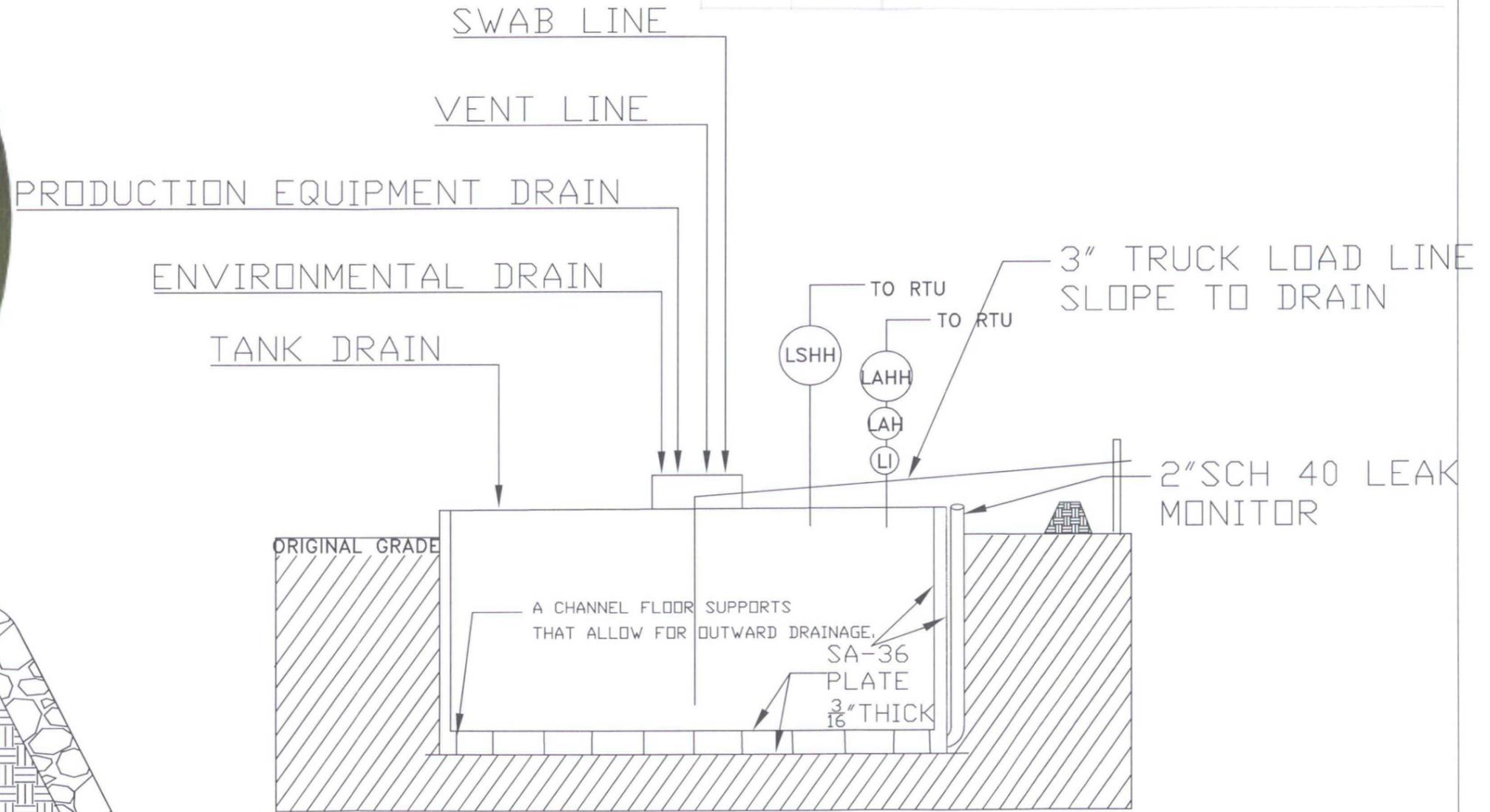
PROPERLY CONSTRUCTED FOUNDATION CONSISTING OF A LEVEL BASE FREE OF ROCKS, DEBRIS, SHARP EDGES OR IRREGULARITIES TO PREVENT PUNCTURES CRACKS OR INDENTATIONS TO THE TANK BOTTOM.
