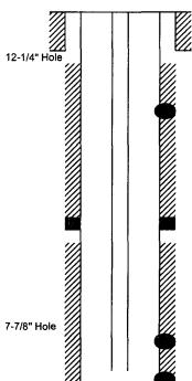
8-5/8" 24# K-55 Casing @ 264' w/ 175 sxs Circulated 15 bbls cement to surface
