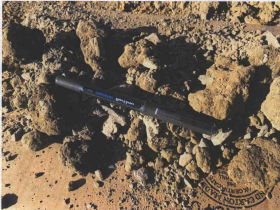
Figure 5: Mixed (3:1) drill cuttings. The soil matrix is approximately 1/3 rock, 1/3 fines, and 1/3 stabilized cuttings.
