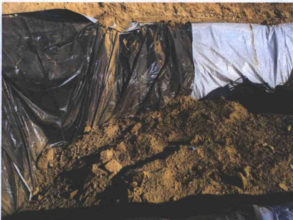
Figure 4: Mixed cutting ratio. 45% stabilized cuttings, 50% fines, 5% rock.
