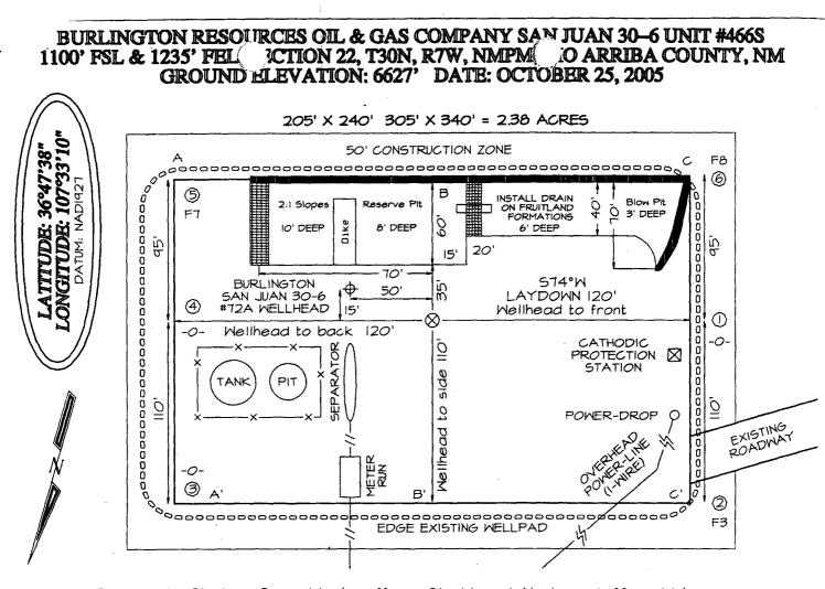
Reserve Pit Dike: to be 8' above Deep side (overflow  $\sim$  3' wide and 1' above shallow side). Blow Pit: overflow pipe halfway between top and bottom and to extend over plastic liner and into blow pit.
