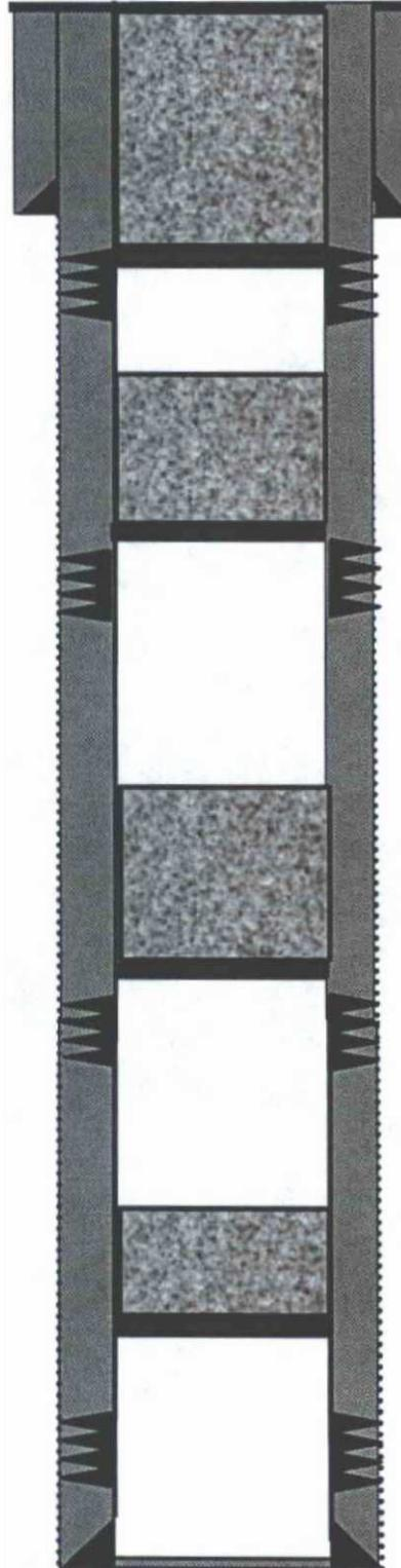
**Plug #4** - Set cement from 153 ft to surface with 60 sks of cement. Circulate to surface. (60 sks of Class G Neat)
