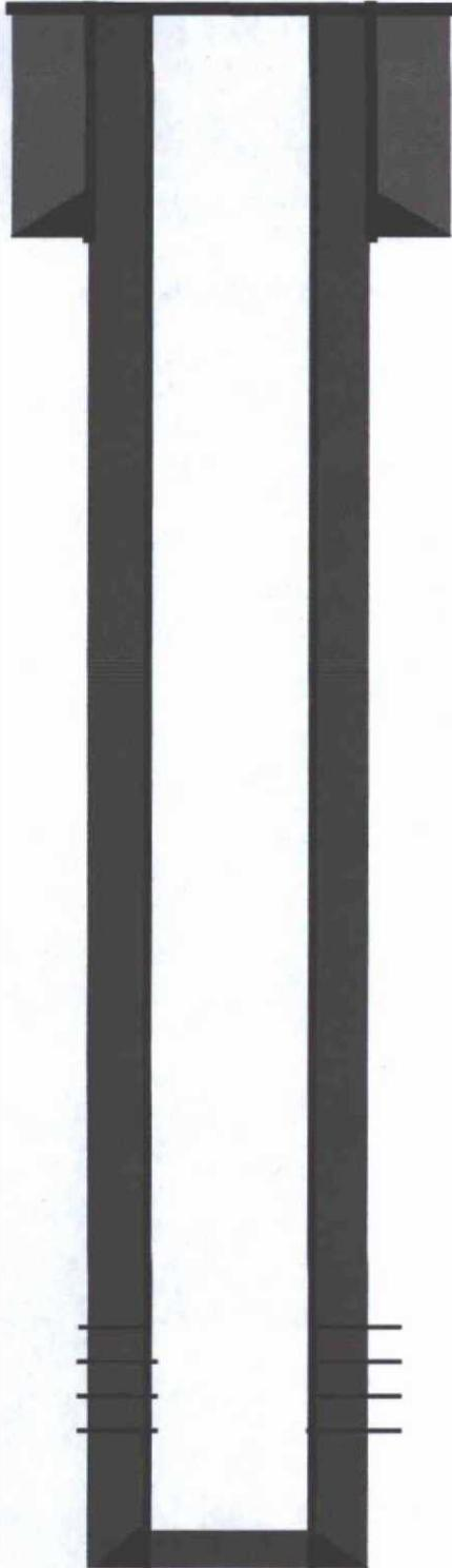
7" J-55 20# casing @ 134'. Cemented with 60 sks Class B w/ 2% gel. Circulated 3 bbl cement to surface
