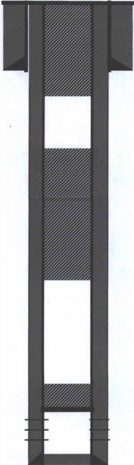
7" J-55 20# casing @ 134'. Cemented with 60 sks Class B w/ 2% gel. Circulated 3 bbl cement to surface. Hole size 8-3/4"
