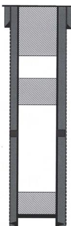
TD 3360° PBTD 3318" 5.5" casing; cement circulated to surface
