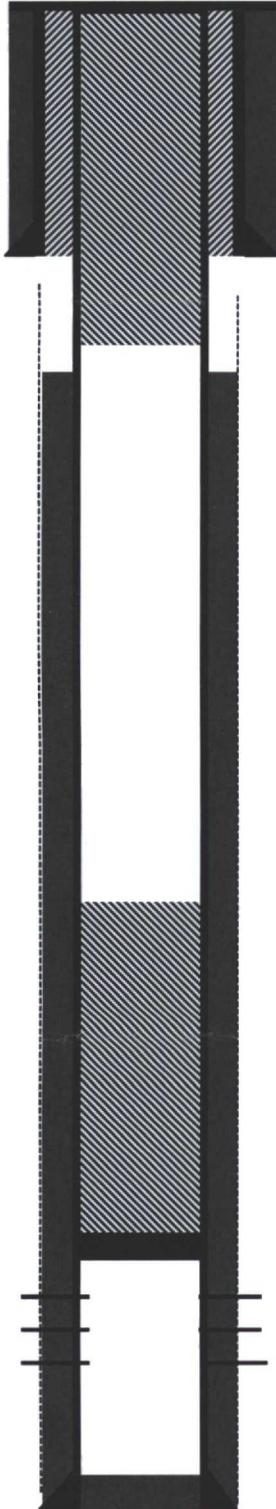
7" 20# ST & C casing @ 92'. Cemented w/ 35
