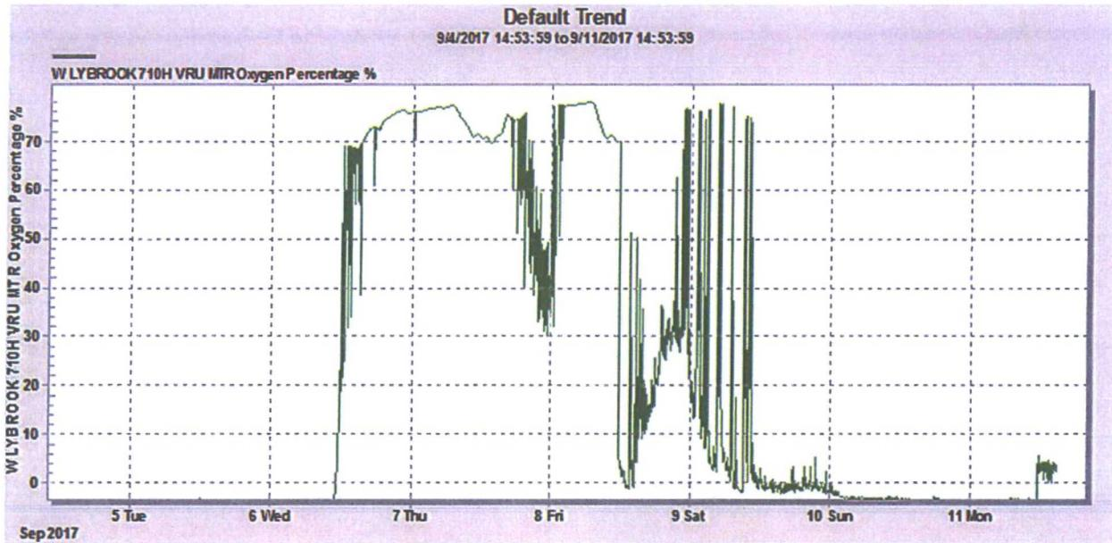
Oxygen Level decreased-9/11/17 but extended the Flare extension due to the workover on the 752H
