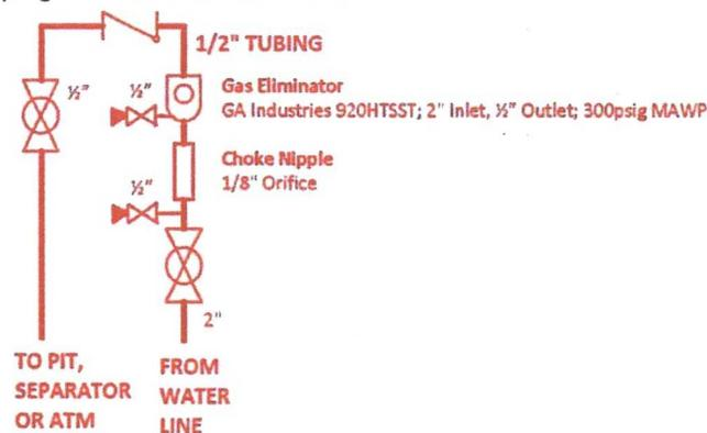
6. Install gas eliminator at the **DAWSON LS 001-MV**. Connect gas eliminator to buried 3" poly water line. Mount box with catalytic heater over water line and gas eliminator. Route the gas eliminator vent line to the Tank Down comer.
