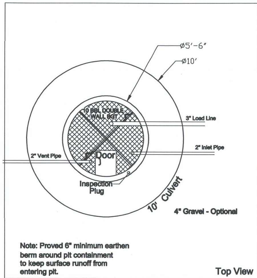
**Note:** Outer edge of BGT will be left open and unobstructed to allow for visual inspection of secondary containment for evidence of leaks.
