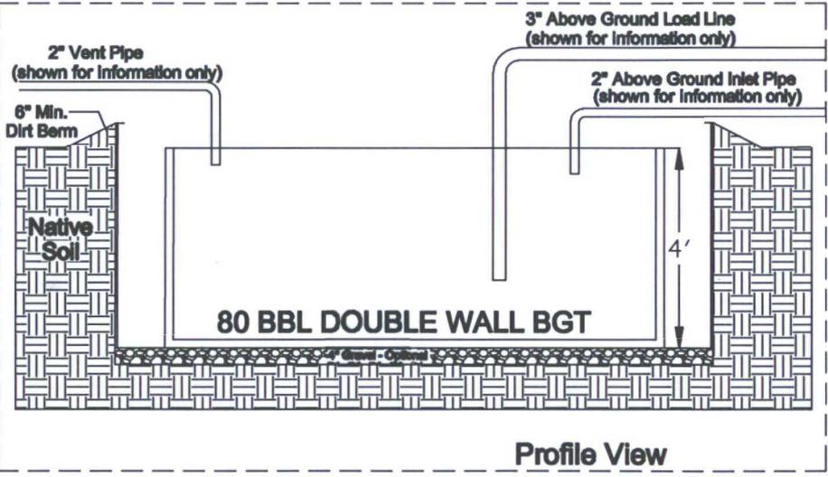
Note: Proved 6" minimum earthen berm around pit containment to keep surface runoff from entering pit.
