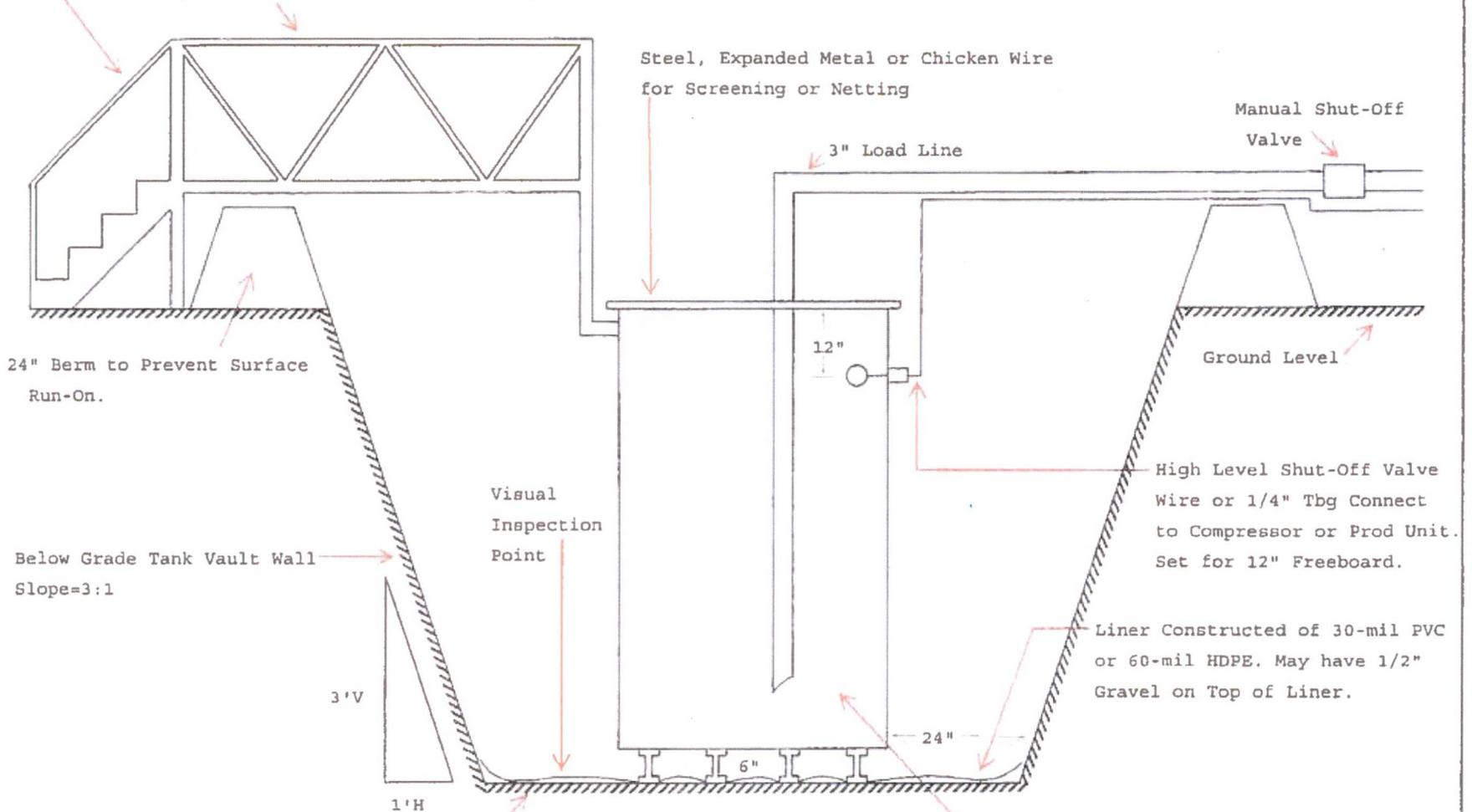
Below Grade Tank Vault-Firm, Level Foundation Free of Rocks, Debris or Irregularities. Slope of Vault Walls Will Be 3'-Vert/1'-Horiz. Dependent on Soil Conditions, 2" x 12" Pre-Treated Lumber will be used as needed to insure integrity of vault walls.
