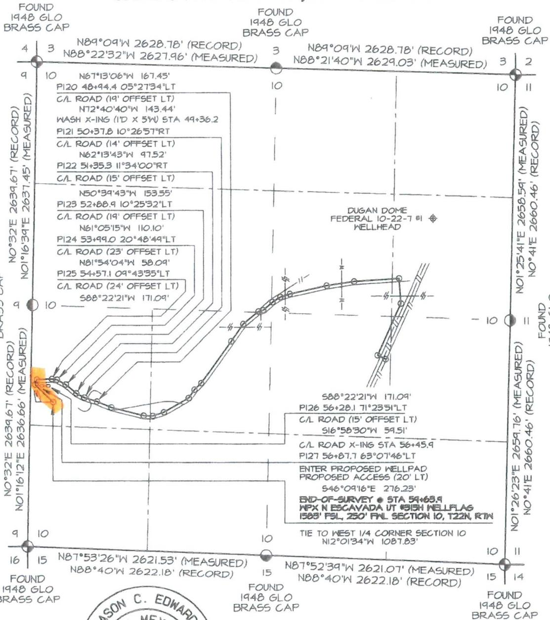
REAL-TIME KINEMATIC GPS SURVEY SOLUTION OBTAINED FROM SATELLITES TRACKED ON JULY 28, 2015 FROM A REFERENCE STATION POSITIONED IN SE/4 NW/4 OF SECTION 2, T22N, R7W
