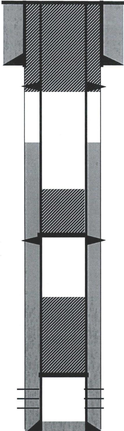
8-5/8" J-55 24# casing @ 141'. Cemented with 100 sks Cement.
