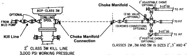
Figure 1 - Drilling Operations - BOP Stack, Choke Manifold and Kill Line Installation for 3,000 psia Pressure Applications
