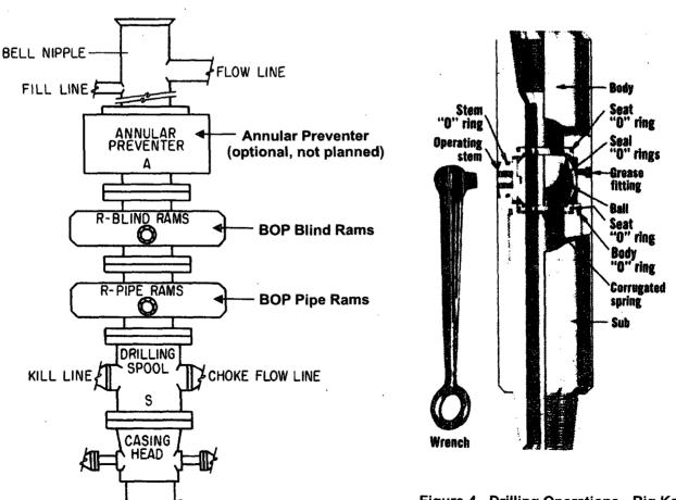
Figure 3 - Drilling Operations - BOP Stack, Choke Manifold and Kill Line Installation for 3,000 psia Pressure Applications
