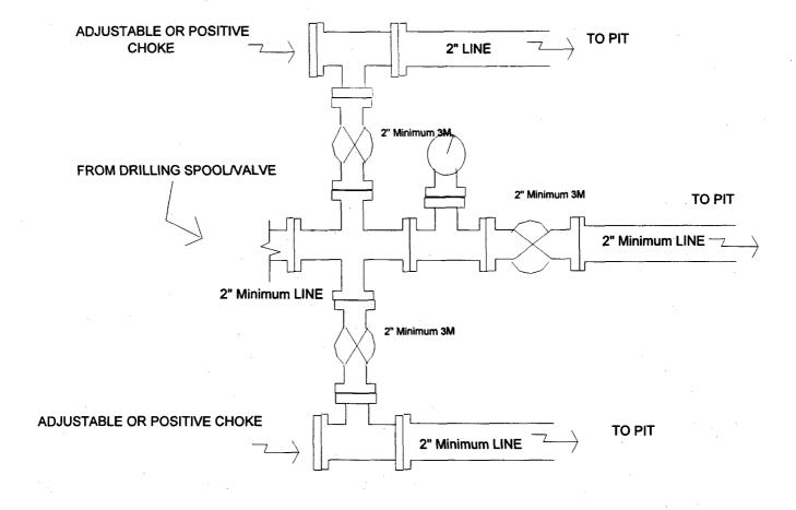
Choke manifold installation from Surface Casing Point to Total Depth. 3,000 psi working pressure equipment with two chokes.
