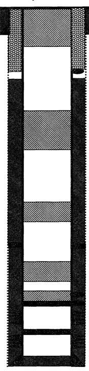
TD 7300' PBTD 7201' 9.625" 36# Casing set @ 475' 250 sxs cement, circulated to surface
