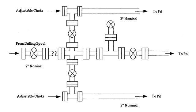
Choke manifold installed from surface to TD
