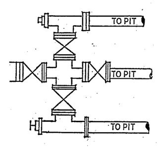
Kill line will be minimum 2" diameter and have 2 valves, one of which shall be a minimum 2" check valve.
