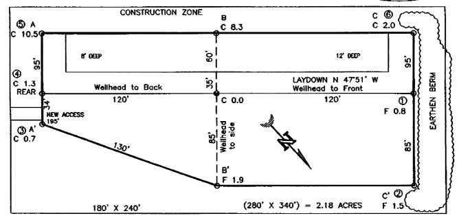
RESERVE PIT DIKE: TO BE 8' ABOVE DEEP SIDE (OVERFLOW - 3' WIDE AND 1' ABOVE SHALLOW SIDE). BLOW PIT: OVERFLOW PIPE HALFWAY SETWEEN TOP AND BOTTOM AND TO EXTEND OVER PLASTIC LINER AND INTO BLOW PIT.
