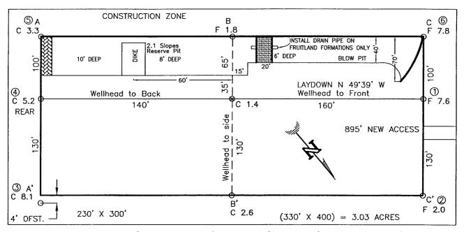
RESERVE PIT DIKE: TO BE 8' ABOVE DEEP SIDE (OVERFLOW - 3' WIDE AND 1' ABOVE SHALLOW SIDE). BLOW PIT: OVERFLOW PIPE HALFWAY BETWEEN TOP AND BOTTOM AND TO EXTEND OVER PLASTIC LINER AND INTO BLOW PIT. NOTE:
