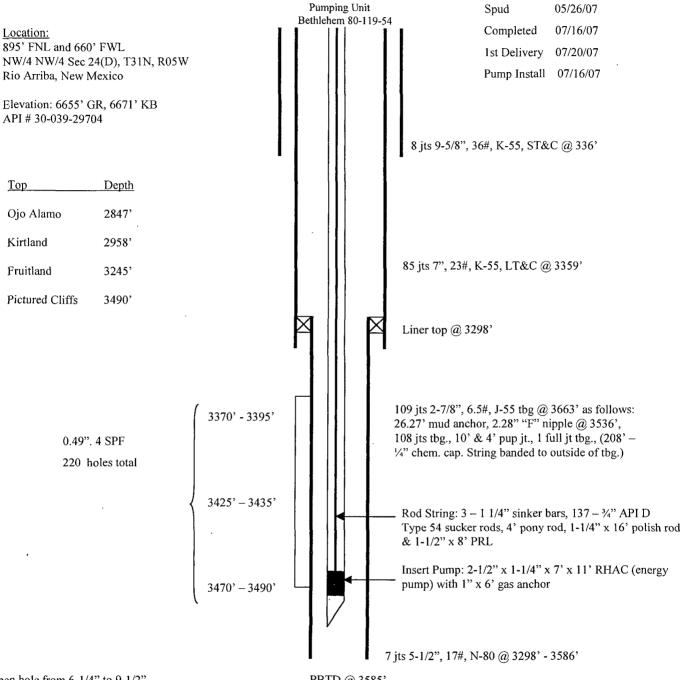
Open hole from 6-1/4" to 9-1/2" from 3369' to 3586'
