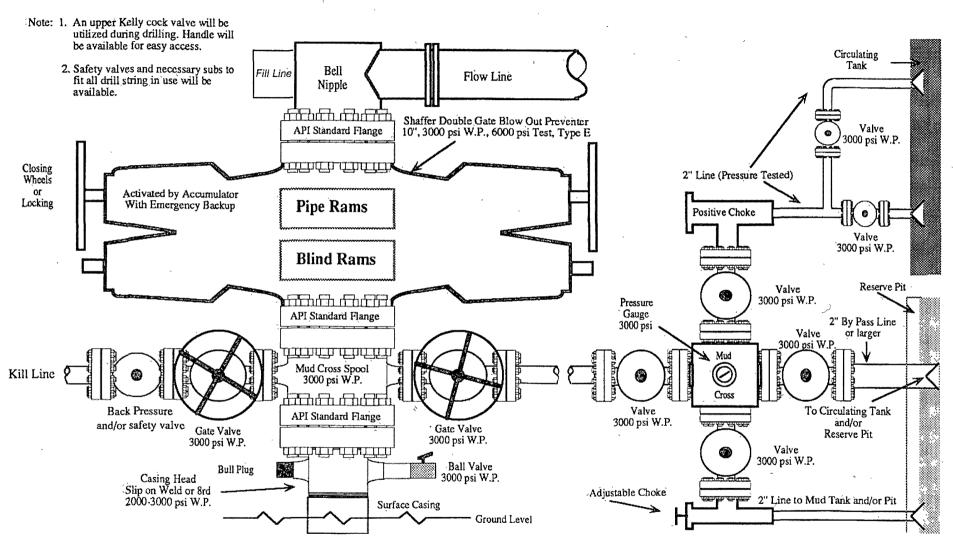
Note: This equipment is designed to meet requirements for a 2-M rating standard per 43 CFR part 3160 (amended). Proper operation and testing of equipment will be carried out per standard. 2,000 psi equipment can be substituted in the drawing to meet minimum requirements per standard.
