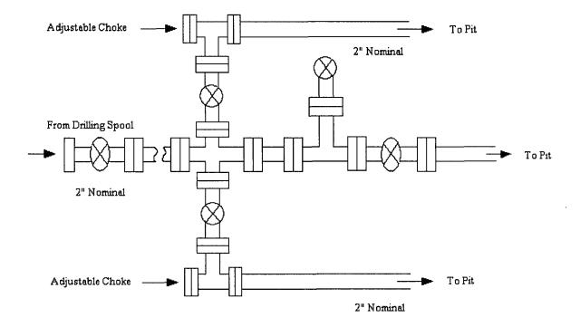
Choke manifold installed from surface to TD
