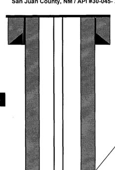
TOC circulated per 75% Calc, and sundry stated show of cement to surface..
