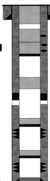
TOC circulated per 75% Calc, and Sundry stated show of cement to surface..
