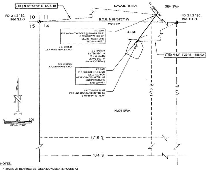
1) BASIS OF BEARING: BETWEEN MONUMENTS FOUND AT THE NORTH QUARTER CORNER AND THE NORTHWEST CORNER OF SEC. 14, T30N, R16W, N.M.P.M. LINE BEARS N 89°38'37" W A DISTANCE OF 2635.23' PER G.P.S. MEASUREMENT.
