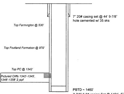
2-7/8" 6.5# casing Set @ 1491', 5" hole TD @ 1509' Cemented w/ 175 sks to surface
