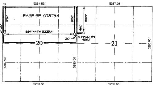
THE HORIZONTAL LATERAL REPRESENTED ON THIS PLAT CORRESPONDS TO THE OLIVE SEGMENT WHICH VARIES IN ELEVATION FROM 7333.0' AT THE POINT-OF-ENTRY TO 7237.0' AT THE END-OF-LATERAL.
