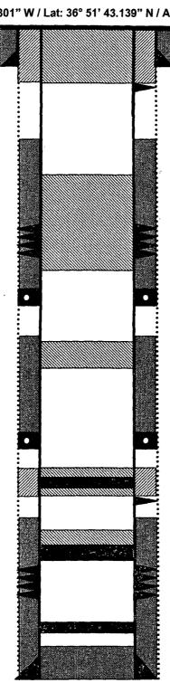
8.625" 32.3# casing set @ 204' Cement with 225 cf, circulated to surface
