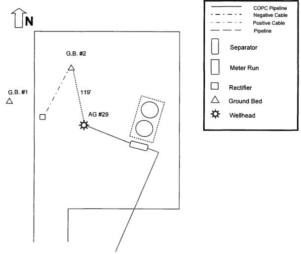
Drill new ground bed approximately 119' North of #29 wellhead at staked location. Run new positive cable from existing rectifier to new ground bed #2 at length listed below.
