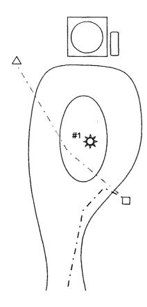
Run new positive cable from existing rectifier to new already drilled ground bed, and plow negative to #191E wellhead at lengths listed below.
