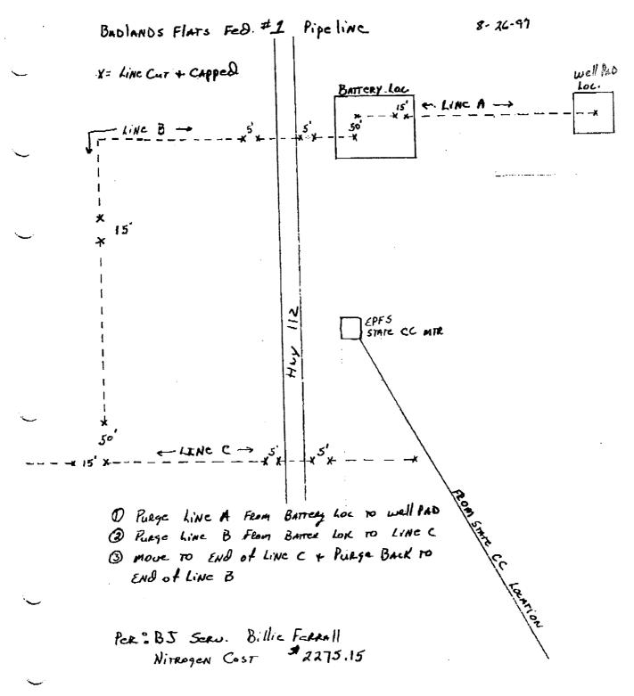
9-12-97 Line from Well Location to Sales Meter Connection was purged with nitrogen.
