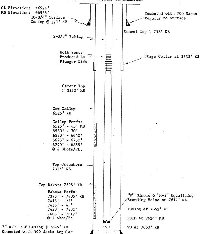
Centralizers Located 10' & 60' Above Casing Setting Depth and 90' Thereafter to 6555' KB; Also One Centralizer 30' Above and 30' Below Stage Collar.
