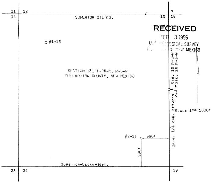
1, W W STUDDERT, REGISTERED PROFESSIONAL ENGINEER No. 388, STATE OF NEW MEXICO, HEREBY CERTIFY THAT THIS WELL LOCATION: SUPERIOR OIL CO., SUPERIOR-SLOAN-GOVT., #2-13, 990' FROM THE SOUTH AND EAST LINES OF SECTION 13, T-25-N, R-6-W, RIC ARRIBA COUNTY, NEW MEXICO, WAS STAKED ON THE GROUND UNDER MY SUPERVISION AND THAT WW STUDGERT THIS PLAT IS TRUE AND CORRECT.
