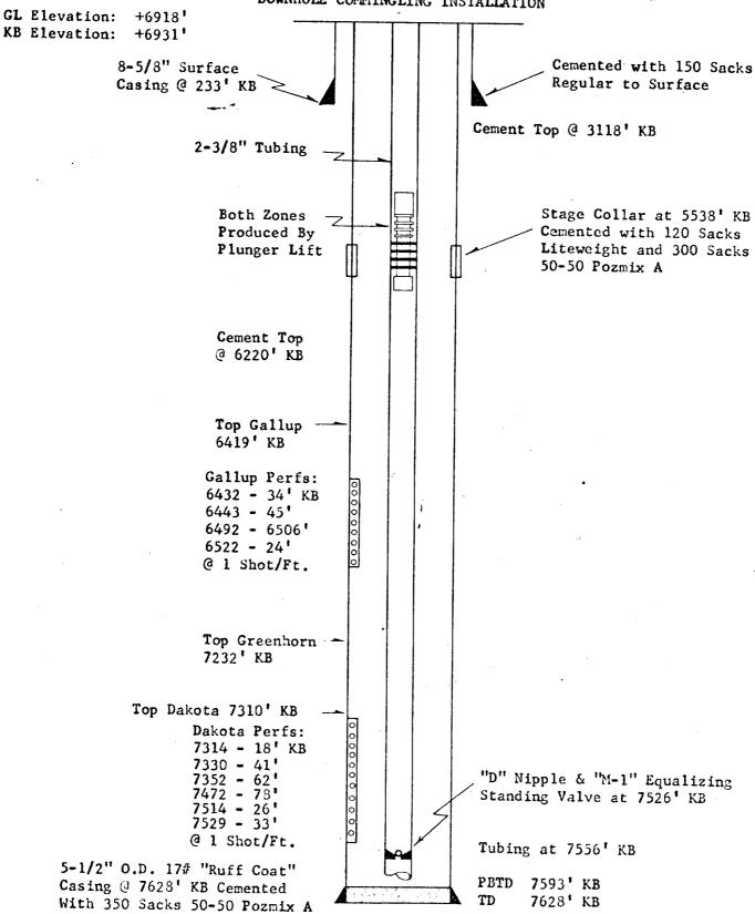
Centralizers Located 10' and 60' Above Casing Setting Depth and 90' Thereafter to 6388' KB; Also One Centralizer 30' Above & 30' Below Stage Collar
